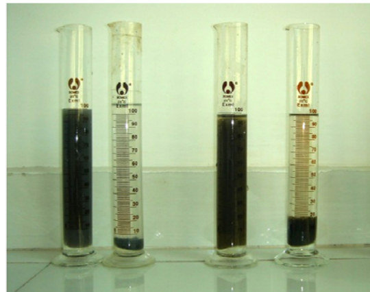
Figure 2: Wastewater treatment samples before and after polyacrylamide application
